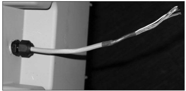
Figure 7.9 - Loosen cable gland and extend the cable out of the gland
