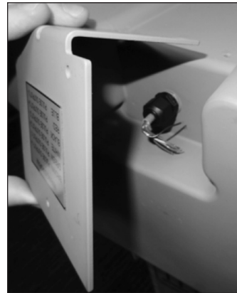
Figure 7.1 - Pulse output cable is covered by a protective plate
