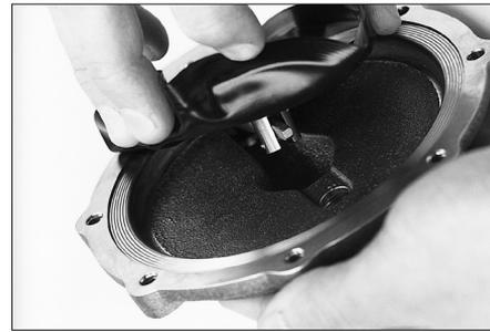
Make sure lever is centered in the diaphragm retainer
