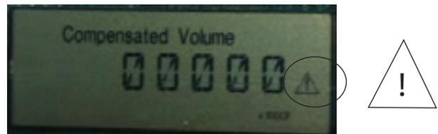
**Figure 10.1**—Fault/Alarm symbol as displayed on LCD Screen
