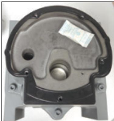
**Figure 8.18**-Interface gasket placed on meter body
