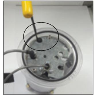
**Figure 11.10**-Remove single screw holding counter to unit
