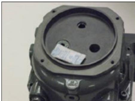
Figure 8.6-New desiccant pack in place
