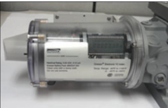
Figure 8.51-Top inlet orientation of AMR bracket
