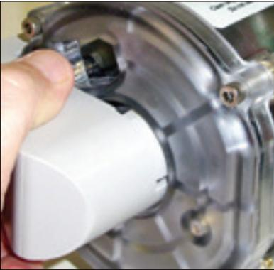
Figure 8.55-Place cable gland connector into recess
