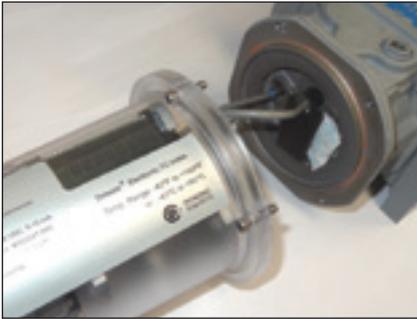
**Figure 8.11**-Seat mag pick-up in magnet well
