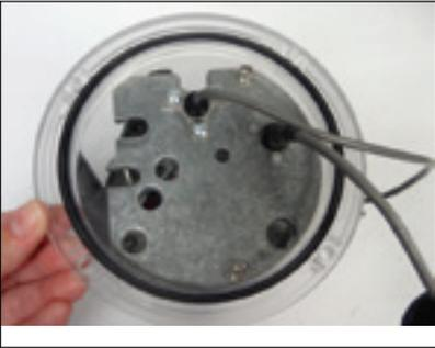
**Figure 8.28**-Orange O-ring seal seated in circular groove
