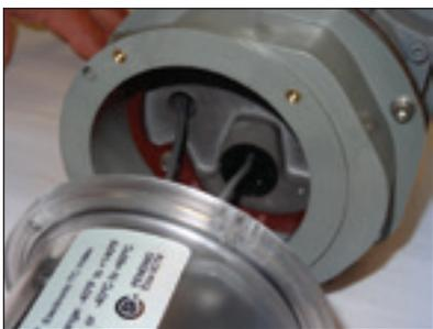
**Figure 8.41**-Seat mag pick-up in magnet well
