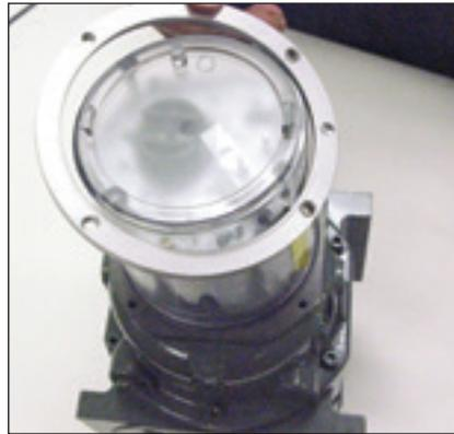
**Figure 8.2-**Remove slip flange
