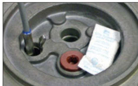
Figure 8.10-Insert temperature probe
