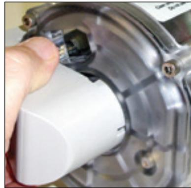
**Figure 8.48**-Place cable gland connector into recess
