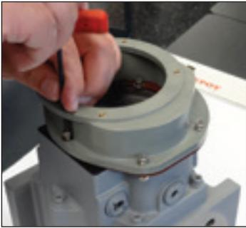
**Figure 8.22**-Install cap screws, washers and hex lock nuts.
