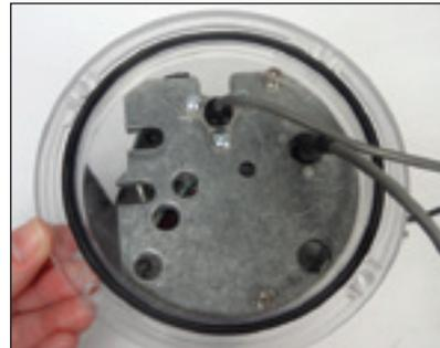
Figure 8.9-Orange O-ring seal seated in circular groove.
