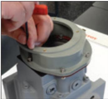
**Figure 8.40**-Install cap screws, washers and hex lock nuts.
