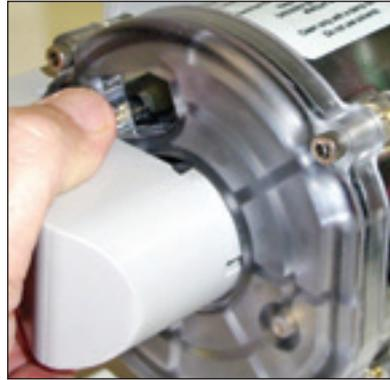
Figure 8.58-Place cable gland connector into recess
