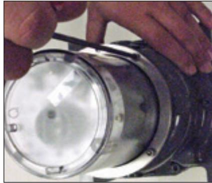
**Figure 8.1-**Remove four hex screws
