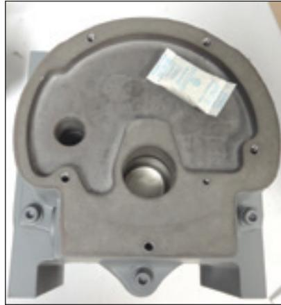
**Figure 8.31**-New desiccant pack in place.
