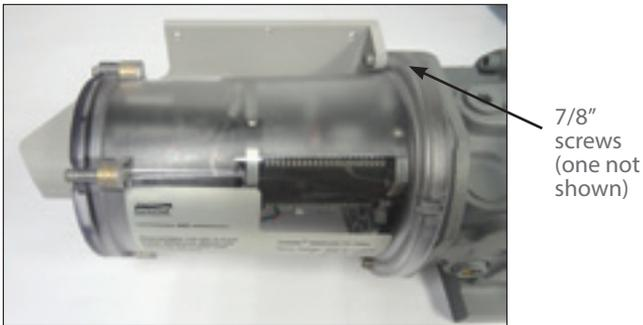
**Figure 8.45**-Insert the 7/8" (long) screws
