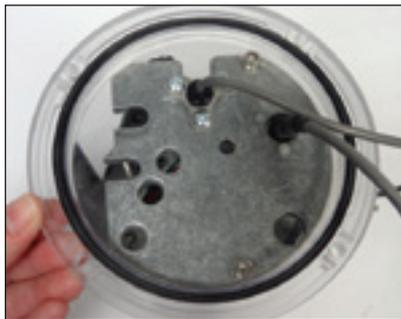
**Figure 8.17**-Orange O-ring seal seated in circular groove
