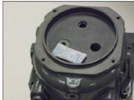
**Figure 8.25**-New desiccant pack in place
