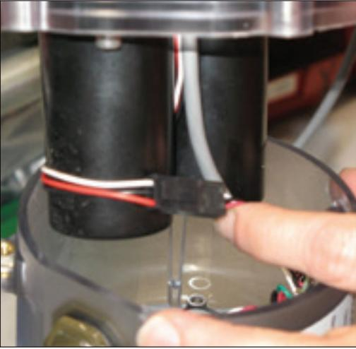
**Figure 11.8**-Remove excess slack: AMR version
