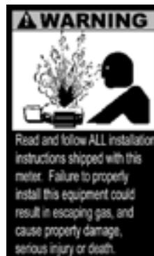
**Danger:** Slowly depressurize and vent all pressure from the meter set before working on the meter.
