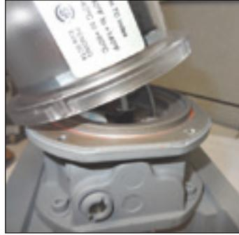
**Figure 8.30**-Seat mag pick-up in magnet well
