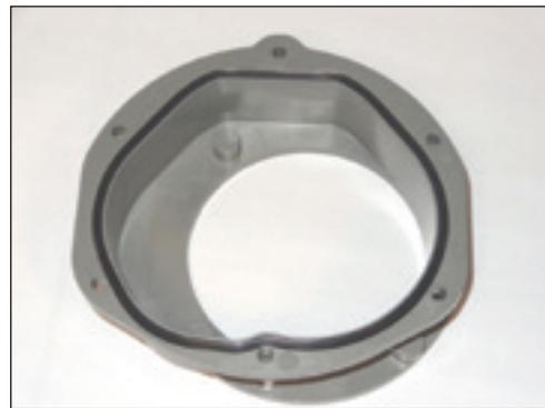
**Figure 8.20**-Quad ring seal seated into groove.
