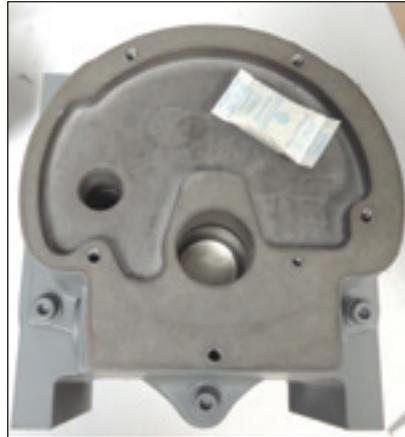
**Figure 8.13**-New desiccant pack in place.
