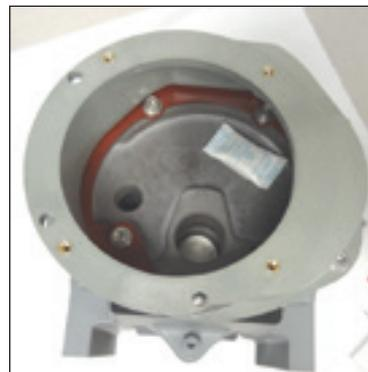
**Figure 8.21**-Lexan Adapter Housing placed on top of the adapter plate.
