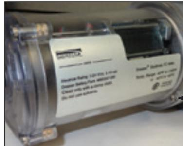
**Figure 8.43**-Insert the 3/4-inch (short) screw
