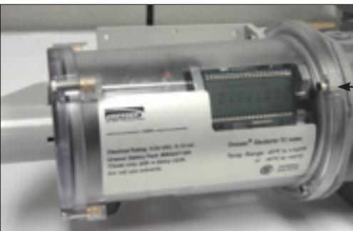
Figure 8.57-Insert the 3/4-inch (short) screw
