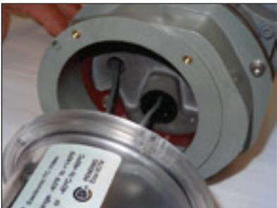
**Figure 8.23**-Seat mag pick-up in magnet well
