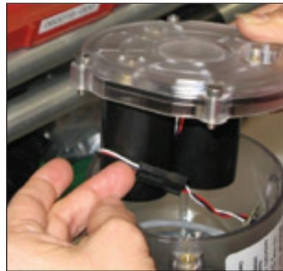
Figure 11.3-Remove excess slack: circular version
