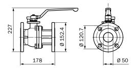
Ball valve, 2" version for high temperatures
