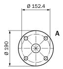
Sender/receiver unit (digital) with electronic unit for ATEX zone 2: Nominal length 220 mm for pipe diameters up to 48"; nominal length 350 mm for pipe diameters > 48" to 72"
