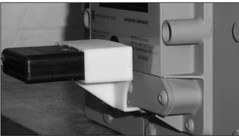
Figure 15 - IrDA adapter placed into slot
