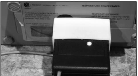
Figure 17 - Light indicating connection established
